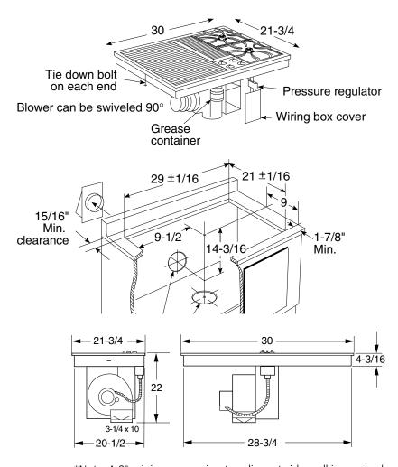
\*Note: A 8" minimum spacing to adjacent side wall is required
